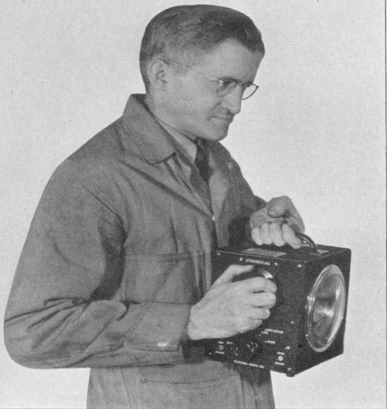
FIGURE 2. The controls and the scale of the Strobotac are arranged for maximum convenience. When the instrument is held in the left hand, as shown, the right hand is used to adjust the speed, which is read directly from the scale on the top of the case.
